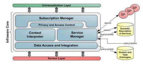
Fig. 1. The Infraware platform's general architecture
