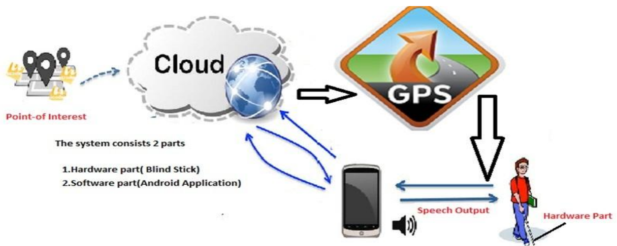
Fig 1: Proposed Architecture to Assisting Mobility for the VI using IoT Infrastructure.
