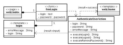
Figure 4. Navigation model for the Login scenario of Authenticate User use case (Portal LabES).
