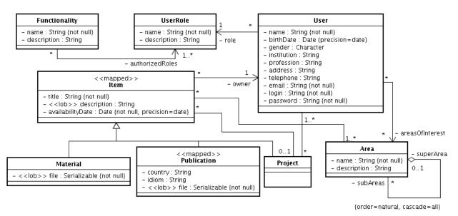
Figure 3. Domain model for the User Management module of LabES Portal.
