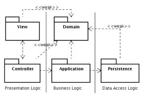
Figure 2. FrameWeb's standard architecture for WebApps
