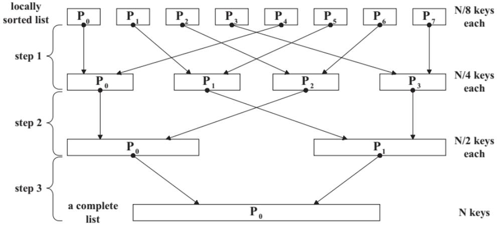
Fig. 1. Conventional parallel merge sort with 8 processors.
