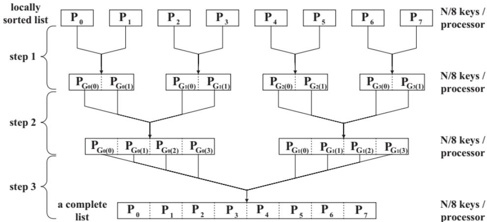
Fig. 2. Load-balanced parallel merge sort.
