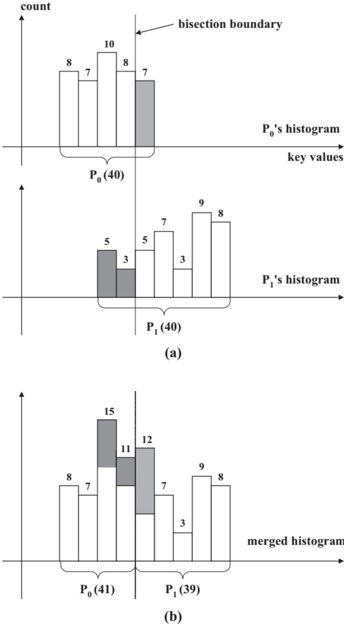
Fig. 3. Example of exchanging and merging keys by using histogram at first iteration (Processors  $P_0, P_1$  both have 40 keys before merge, and 41 & 39 after merge, respectively.) [(a) before merge, (b) after merge].
