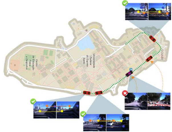
Fig. 1. Illustration of VIBML performing global localization and position tracking around the UFES' campus. VIBML uses previously learned image-pose pairs stored in a neural map to estimate global poses (red cars) from currently observed images. VIBML's neural position tracking keeps a smooth trajectory (green dots), even in case of global localization failure (purple car).
