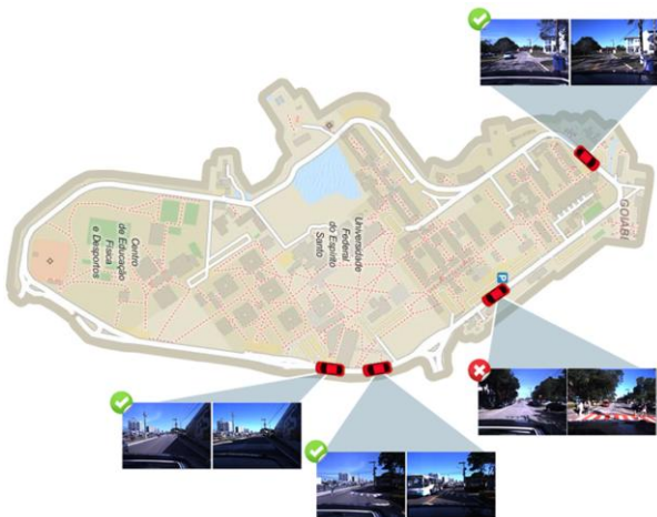
Fig. 1. Examples of VibGL results for a full lap around the Universidade Federal do Espírito Santo (UFES). Images on the left and right of each image pair are samples of images received as input and returned as output by VibGL respectively. Red cars denote the poses estimated by VibGL. Green-marked images are samples of true-positives image-pose pairs outputted by VibGL, while the red-marked one is a sample of a false-positive.
