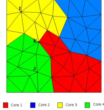
**Fig. 1.** Example of the partitioned mesh with 4 subdomains.
