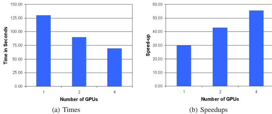
**Fig. 4.** BOXX Personal Supercomputer times and Speedups.
