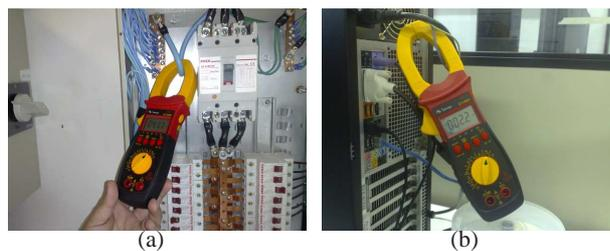
**Fig. 6.** Power (current) measurement setup. (6(a)) Cluster setup: the total current consumed by Enterprise 3 was measured on the neutral wire of its power distribution panel. (6(b)) BOXX Personal Supercomputer setup: the total current consumed by it was measured on the neutral wire of its power cord.
