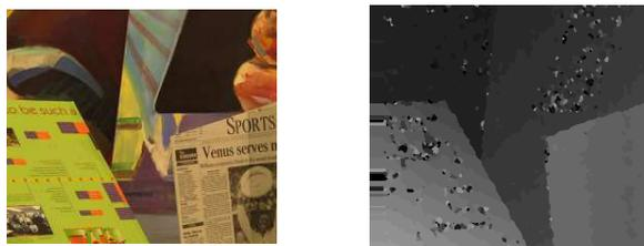
Figure 8: Right image of the stereo pair and the disparity map generated by the best VG-RAM WNN architecture configuration using the "Venus" stereo image pair.
