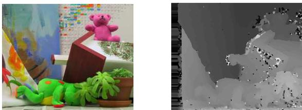
Figure 9: Right image of the stereo pair and the disparity map generated by the best VG-RAM WNN architecture configuration using the "Teddy" stereo image pair.
