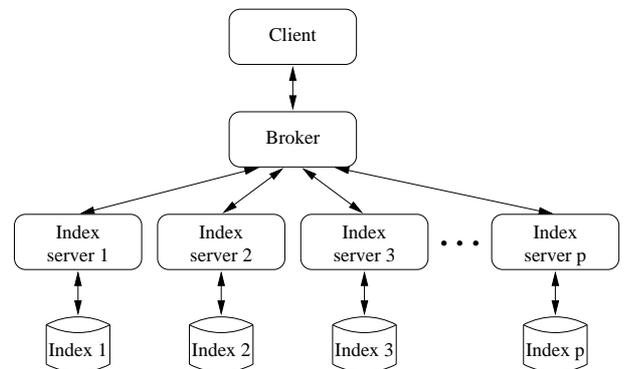
Figure 1: Architecture of a typical search engine.
