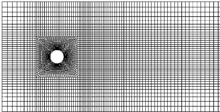
Figure 14. Finite element mesh with 4683 nodes and 4520 elements.
