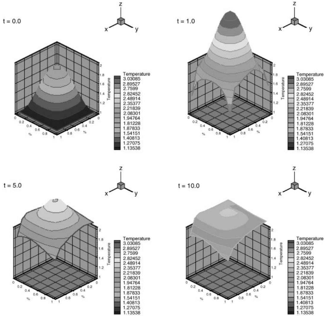
Figure 18. Evolution of temperature solution using bilinear elements on a  $8 \times 8$  grid for the non-isothermal problem.
