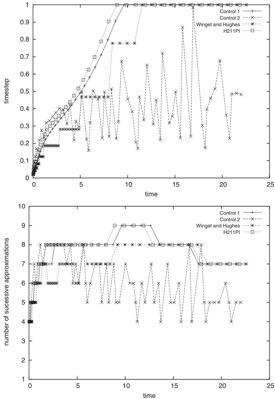
Figure 11. Timestep variation (top) and number of successive approximations (bottom) using Control 1, Control 2, W&H and H211PI for  $Re = 100$ .
