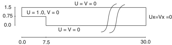
Figure 8. Backward-facing step geometry with channel dimensions and boundary conditions.
